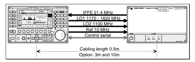
Assembly is very easy. There are no changes in the existing ESMC (apart from any firmware update, if required). Just unpack the frequency extension and cable set, connect them with the ESMC, plug in power cord and antenna cable, that's it.
